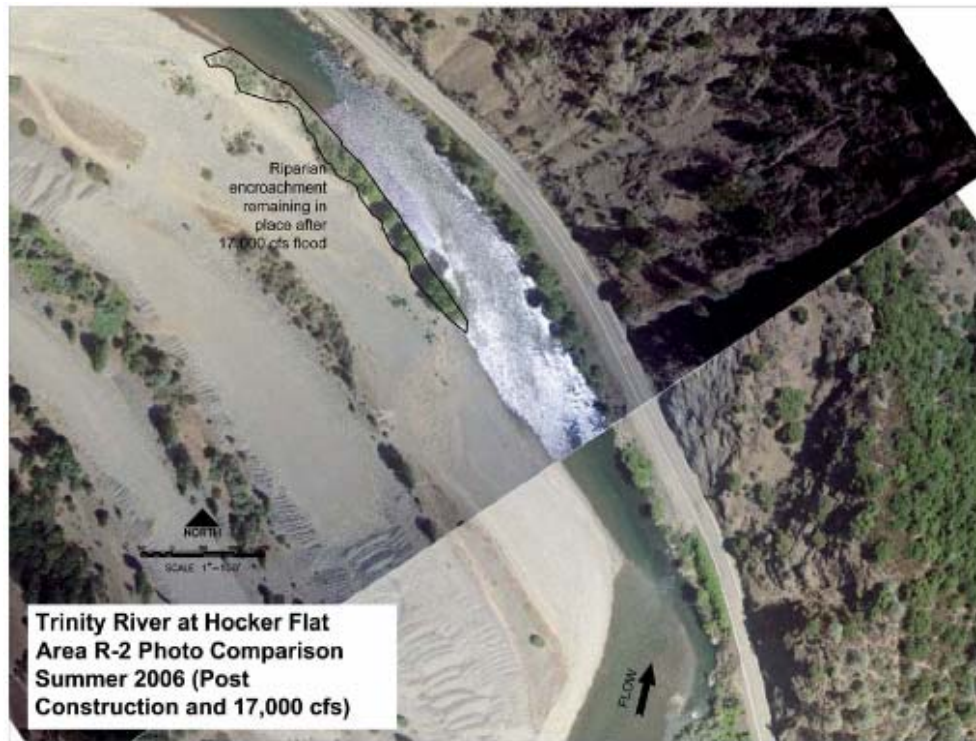
Figure 6. Trinity River at Hocker Flat, post-construction, and post 17,000 cfs flow. Note that riparian encroachment remains in place despite being fully exposed to high flows that are greater magnitude than maximum ROD releases (11,000 cfs).
